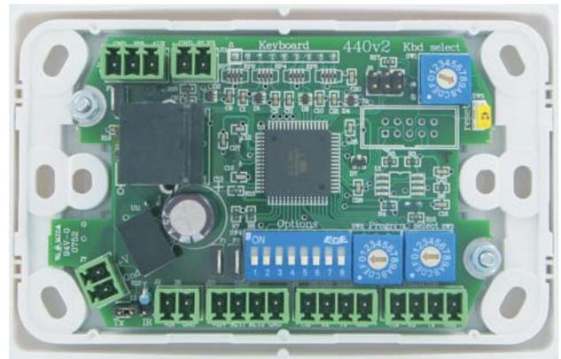
Just below this input connector is a CAT5 socket. This is a quick wiring option for the communications/power/PIR to the T447 "cable-top" box which provides terminations to the projector (DB9), power in socket, and PIR screw terminals. (It is NOT an Ethernet connection.)
