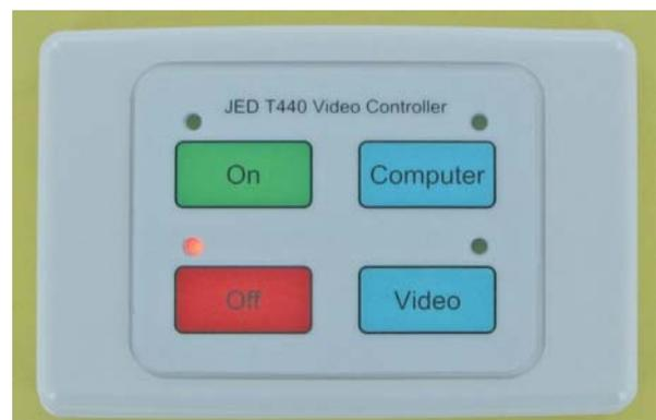
The particular channel LED is ON from the start of warm-up, and it blinks and then continues to show the current channel;
